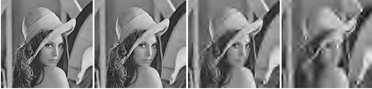
Figure 6: Image quality at 0.2 bpp total rate for unequal erasure protection on a channel with an exponential loss model that averages 20%. Loss rates from left to right: 30%, 40%, 50%, and 60%.
