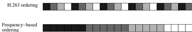
Fig. 4. H.263 bit stream layout and frequency-based bit stream layout. The darker colors represent data that are more important to the quality of reconstruction.
